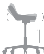
Tilting mechanism / Gas lift
