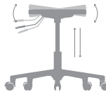
Balance360° mechanism / Gas lift
