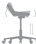
Tilting mechanism / Gas lift
