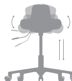
Balance360° mechanism / Gas lift
