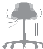
Balance360° mechanism / Gas lift
