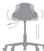
Balance360° mechanism / Gas lift
