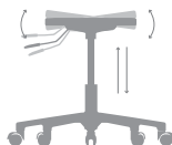
Balance360° mechanism / Gas lift
