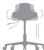
Balance360° mechanism / Gas lift
